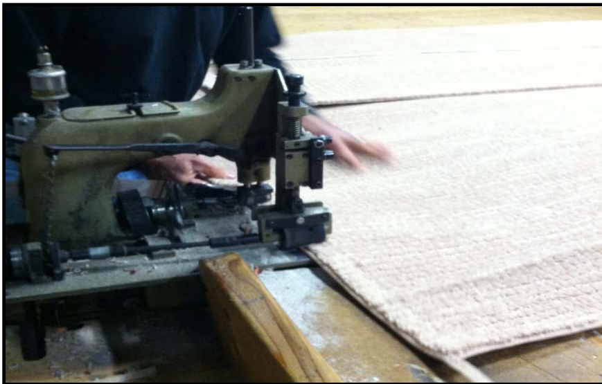
CARPET BEING BOUND IN THE WORKROOM FOR INSTALLATION ON STEPS
